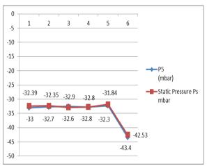
Graph20: Average P5 = -34.47 m bar Avg Static Pressure (PS) = -34.13 m bar
