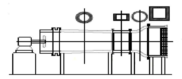
Figure No: 1 LINE SKETCH OF A WIND TUNNEL
