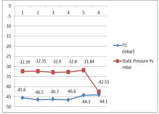
Graph17: Average P2 = -45.57 m bar Avg Static Pressure (PS) = -34.13 m bar
