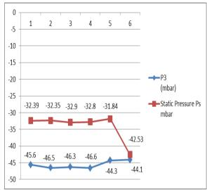
Graph18: Average P3 = -45.57 m bar Avg Static Pressure (PS) = -34.13 m bar
