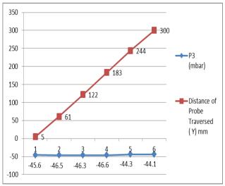
Graph23: Average P3 = - 45.57 m bar Avg Distance of Probe = 152.5 mm
