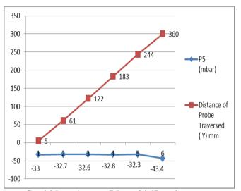
Graph25 : Average P5 = - 34.47 m bar Avg Distance of Probe = 152.5 mm
