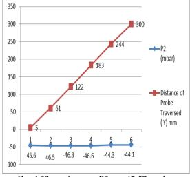
Graph22: Average P2 = - 45.57 m bar Avg Distance of Probe = 152.5 mm
